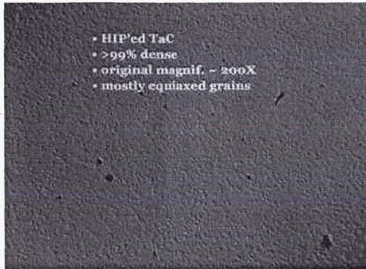
Figure 3 – HIP'ed TaC, as polished. (Courtesy of Exothermics, Inc.)
